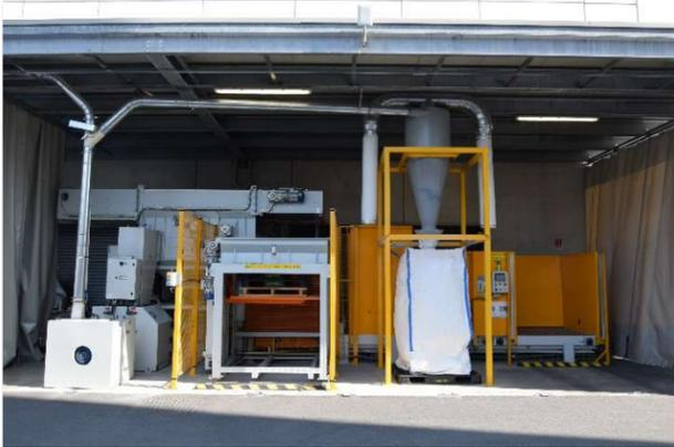
Bag emptying coefficients increase with an emptying mechanism through rotating blades and mixers. Subsequently, a gravimetric fall ensures the separation of most of the material from the bag, released by a counter comb. The pallet loading takes place through a forklift. After the emptying cycle is done, the empty pallet is removed by the forklift. Greater automation can be achieved by integrating an empty pallet stacker and a full pallet accumulator.
